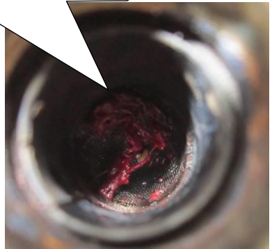
The filter is blocked by impurity, the suction of the compressor will be affected
