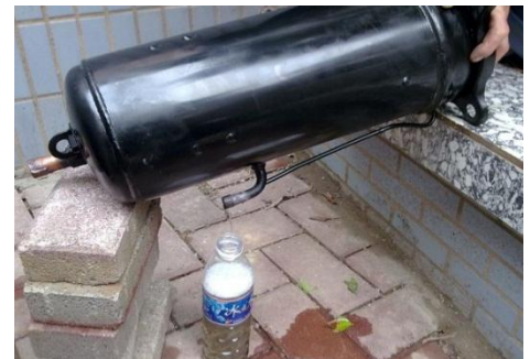
Figure 5-4.14: Draining oil from a compressor
