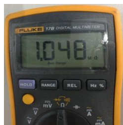
Figure 5-4.6: Measuring resistances among compressor terminals
