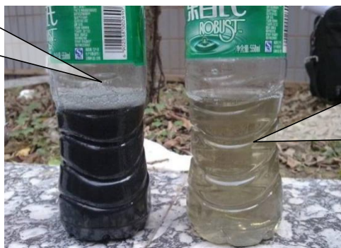
Figure 5-4.16: Inspecting compressor oil
