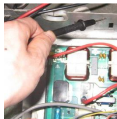
Figure 5-4.7: Measuring resistances between compressor terminals and ground
