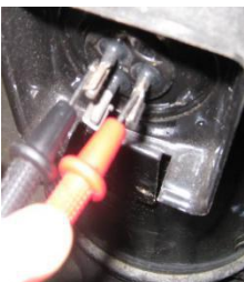
Figure 5-4.6: Measuring resistances among compressor terminals
