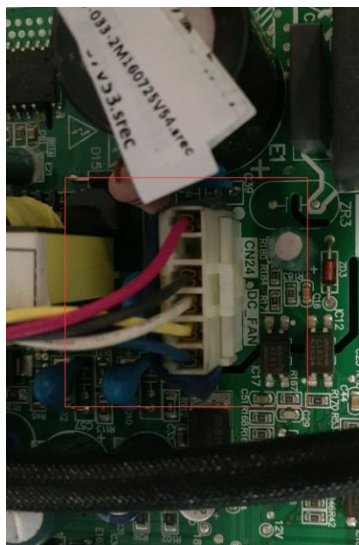
Figure 5.1: Fan connection wiring on indoor unit main PCBs
