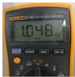
Figure 5-4.6: Measuring resistances among compressor terminals
