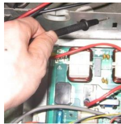
Figure 5-4.7: Measuring resistances between compressor terminals and ground
