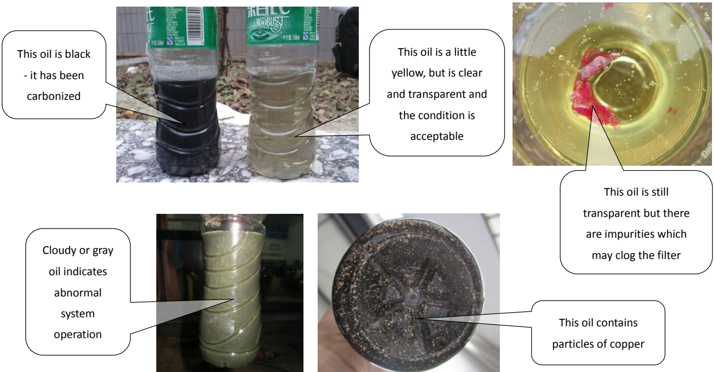
Figure 5-4.16: Inspecting compressor oil
