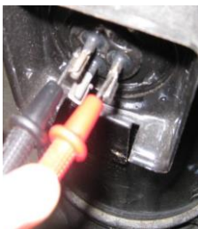
Figure 5-4.6: Measuring resistances among compressor terminals
