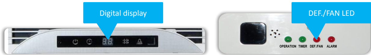
Figure 4-1.3: Indoor unit digital displays and LED indicators
