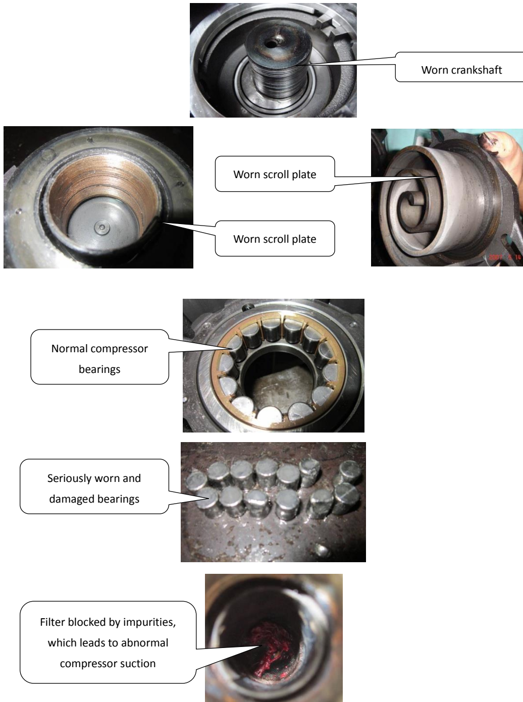
Figure 5-4.17: Effects of spoiled compressor oil
