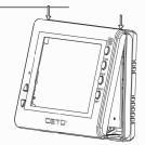
Step 2: Hang the two hooks of the front part at 30° right to the snaps.
