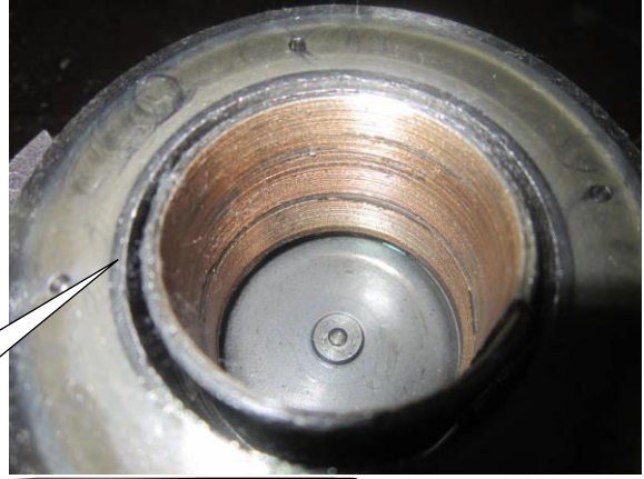
The scroll plate is worn.
