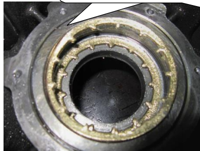
The filter is blocked by impurity, the suction of the compressor will be affected
