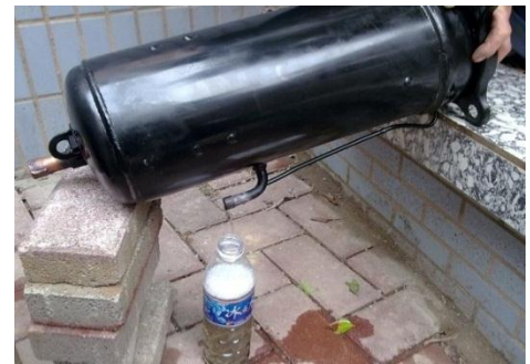
Figure 6-2.5: Draining oil from a compressor
