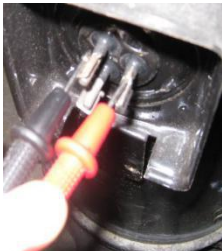
Figure 5-4.6: Measuring resistances among compressor terminals
