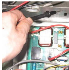
Figure 5-4.7: Measuring resistances between compressor terminals and ground
