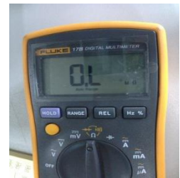
Figure 5-4.7: Measuring resistances between compressor terminals and ground
