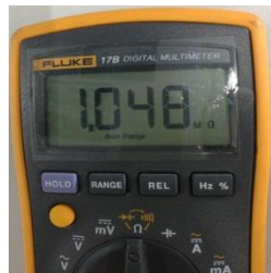
Figure 5-4.6: Measuring resistances among compressor terminals
