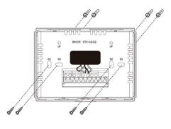
For horizontal mount put one screw left and one screw right.
