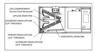
FIGURE 7:Coil Assembly
