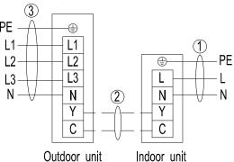
three-phase for cooling only type,380V
