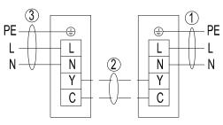
Outdoor unit Indoor unit Single-phase for cooling only type
