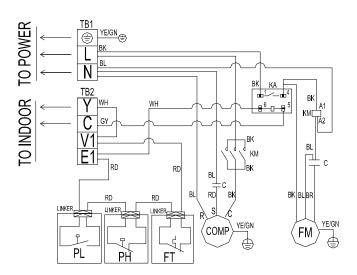
**Suggestion**: The wire diagram is as FIGURE 10 when the outdoor unit is getting feedback from terminals E1, V1.
