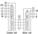
three-phase for cooling and heatpump type,380V
