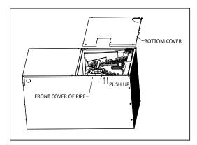
FIGURE 4: Connect the Refrigerant line
