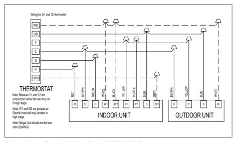
Figure 6 Control Wiring For 18SEER HP Systems
