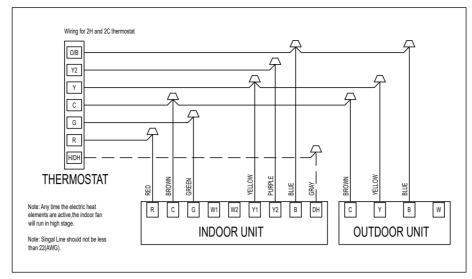
Figure 4 Control Wiring For 18SEER HP Systems
