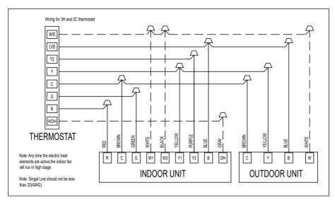
Figure 1 Control Wiring For 18SEER HP Systems
