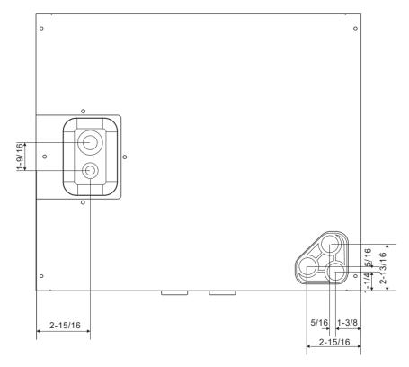
Fig.2 DIMENSIONS FOR FRONT CONNECT COIL
