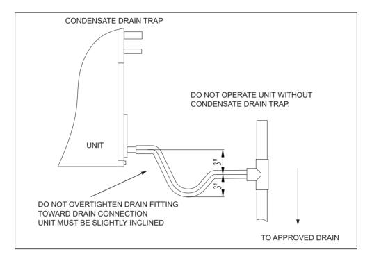
Fig. 3 CONDENSATE DRAIN TRAP
